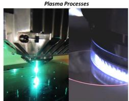
Figuring of nano-Precision Optical Components.
