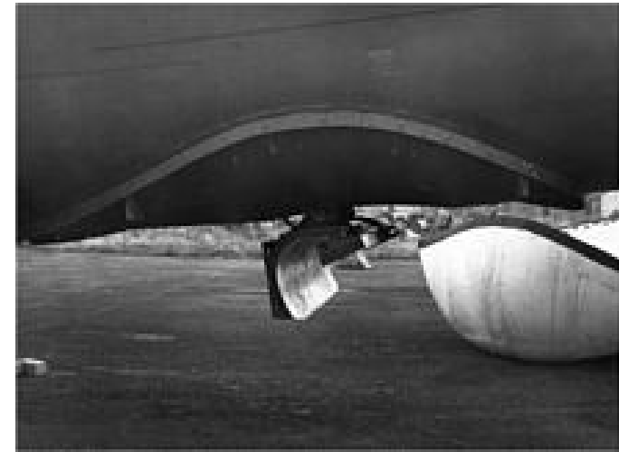
Radar scanner with a waveguide feed and reflector
