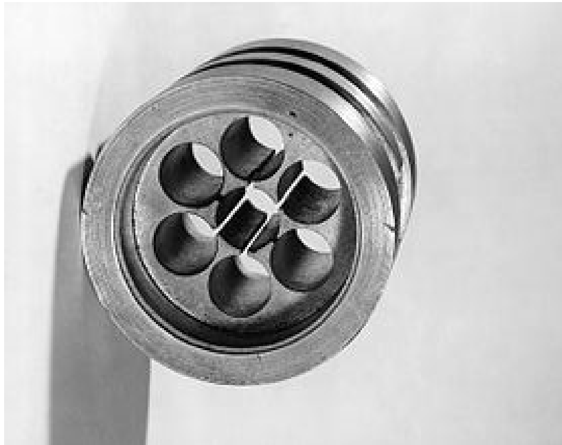
The anode block of an early cavity magnetron showing the initial 6 cavity resonators
