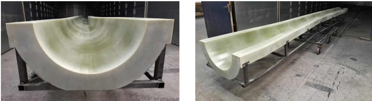
Figure 1: Blade mould half after curing
